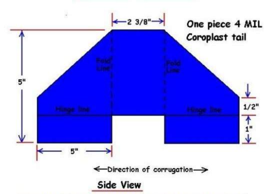
Create hinge by cutting away one side of a coroplast corrugation
