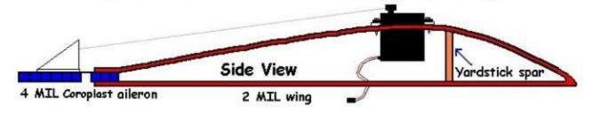
Note: Aileron hinge created by cutting away one side of a Coroplast corrugation
