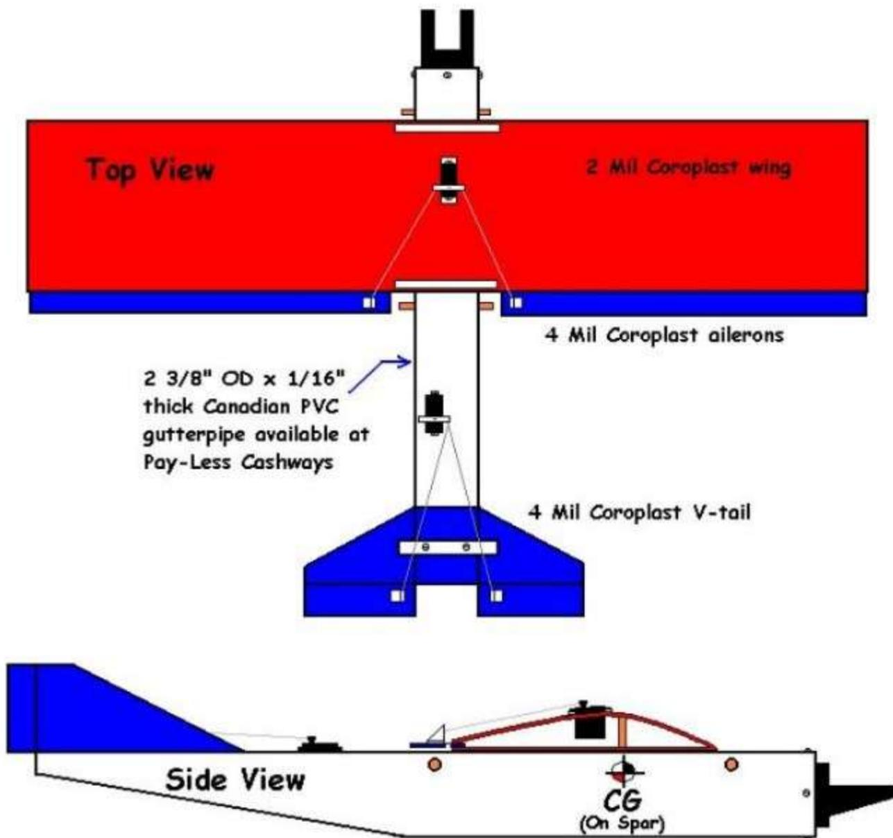
**Note:** V-tail mounted to fuselage with two #6 x 1/2" self tapping screws
