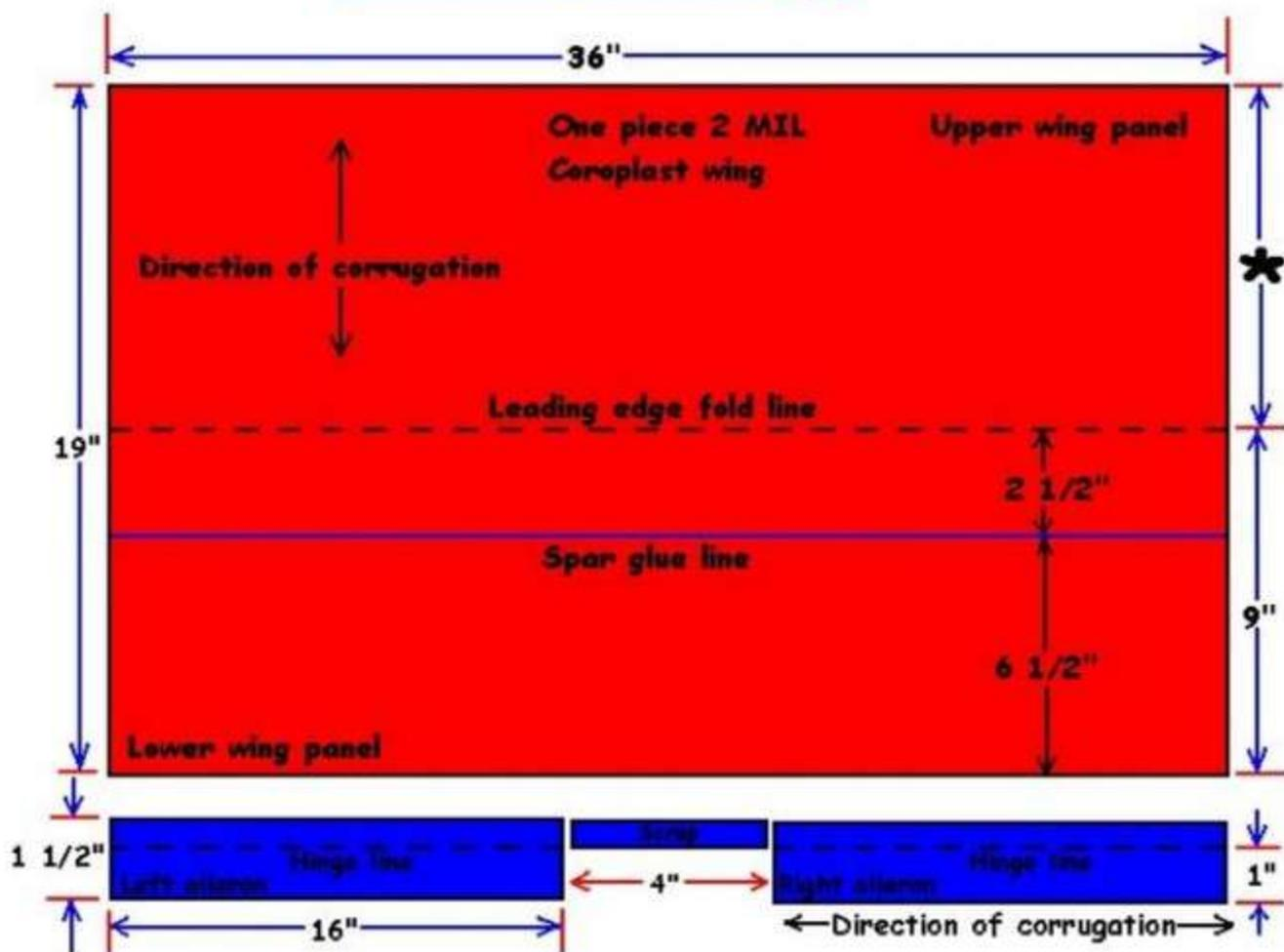
\* This final dimension to be determined during wing building process
