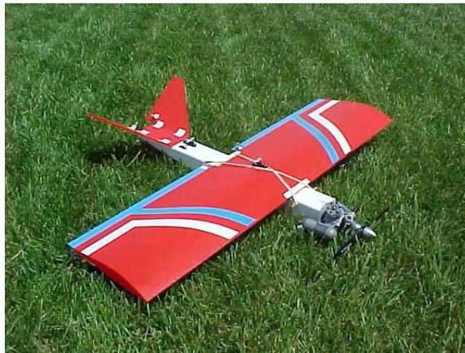
The Derelict. This is our third design entry for an RCCA legal open "B" class plane. The main difference in this design is the choice of materials. We use 2 mil Coroplast® for the wing, and the fuselage is made from a light weight, smaller O.D. gutter pipe. All up flying weight with a Magnum® .25, three Hitec® HS-81 servos and a 270 mah battery is 2 lb 4 oz! The Derelict is our best flying open "B" class design yet, and boy does she fly!
