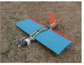
The Defender is our second entry for an RCCA legal open "B" class combat plane. This little "scrapper" has some significant improvements over the Dynamo. The Defender uses standard radio gear and a bearing .25. All out weight comes in at 2 lbs. 12 oz. Flight characteristics are outstanding!
