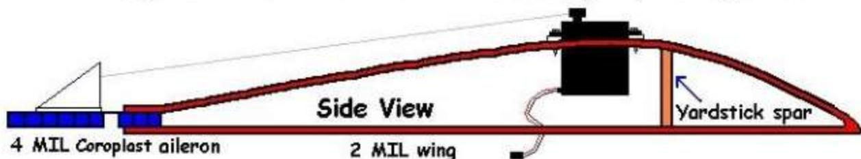
**Note:** Aileron hinge created by cutting away one side of a Coroplast corrugation
