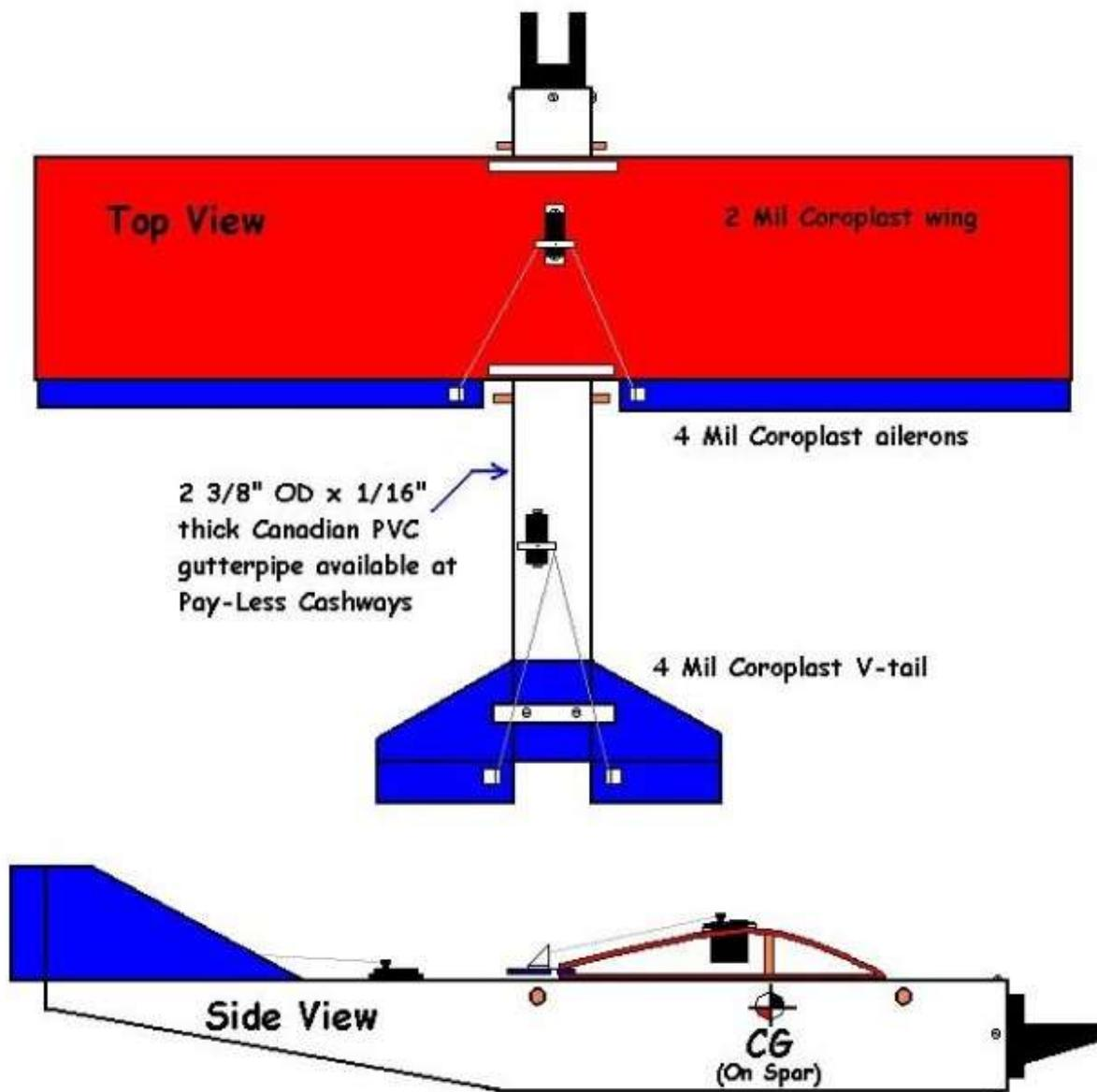
**Note:** V-tail mounted to fuselage with two #6 x 1/2" self tapping screws
