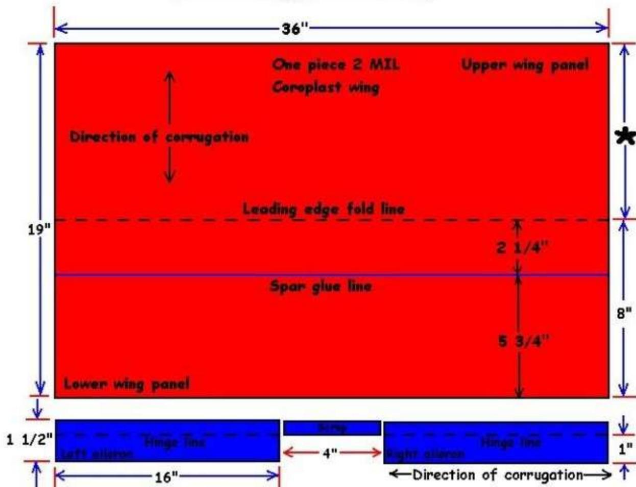
\* This final dimension to be determined during wing building process
