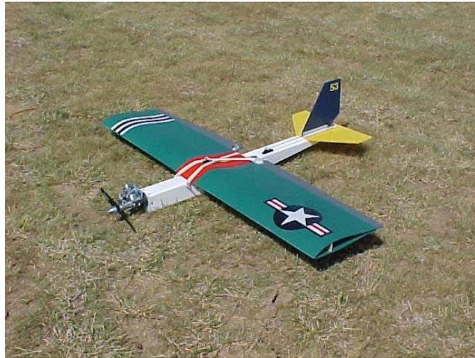
This little gem is named the Debut - and like its name implies - it is designed as an introductory, beginners RCCA open "B" class plane. With a whopping 48" streamer grabbing wingspan, and an all up flying weight of just slightly over 3 lbs (with full size radio gear and a Thunder Tiger Pro .25) this plane is a terrific entry level combat plane that can help you "learn the ropes" of combat!
